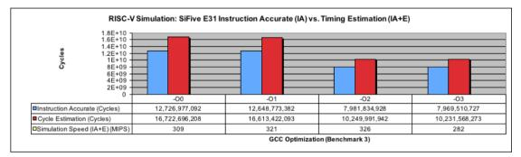
Fig. 6. IA+E cycle estimation results for the SiFive E31 processor.
