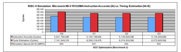
Fig. 5. IA+E cycle estimation results for the Microsemi Mi-V RV32IMA processor.
