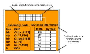
Fig. 2. Simplified view of the timing estimation mechanism.
