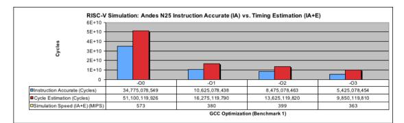
Fig. 4. IA+E cycle estimation results for the Andes N25 processor.
