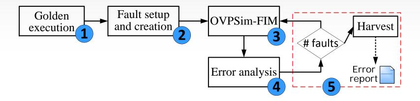
This flow is supported in gem5 and OVPsim simulators
