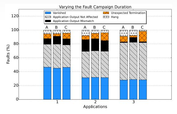
Small deviation in fault detection error between Cycle Accurate (gem5) and Instruction Accurate (Imperas) simulations (A vs. C, B vs. C)
